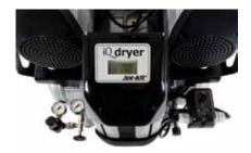
Q2 adsorption dryer mounted on compressor
