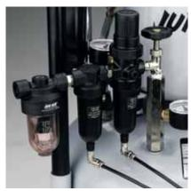
Filters mounted on a compressor
