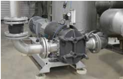
ONIXline pump for conveying C starch
